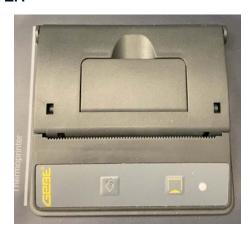
Integrated thermal printer for printing test reports immediately after testing has been completed
